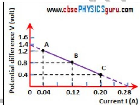
6. Potential difference across terminals of a cell were measured (in volts) against different currents (in ampere) flowing through the cell. A graph was drawn which was a straight line ABC. Using the data given in the graph determine, (i) the emf and (ii) the internal resistance of the cell. [(i) 1.4 V, (ii) 5  $\Omega$ ]
