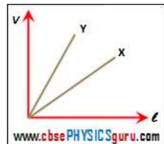
11. The variation of potential difference V with length l in case of two potentiometers X and Y is as shown in the figure. Which one of these two will be preferred for comparing emfs of two cells and why? [X]
