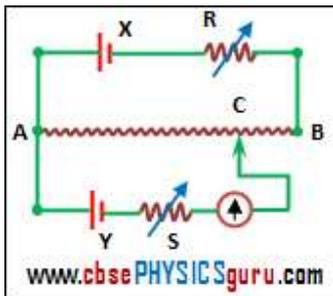
at C. State with reason, where the balance point will be shifted when (1) Resistance R is increased, keeping all parameters unchanged. (2) Resistance S is increased, keeping R constant. (3) Cell X is replaced by another cell whose emf is lower than that of cell Y.
