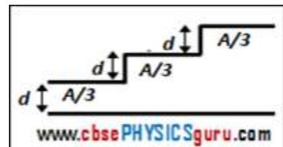
7. Two dielectric slabs of dielectric constants  $K_1$  and  $K_2$  have been filled in between the plates of a capacitor as shown in figure. The capacitance of the capacitor is:
