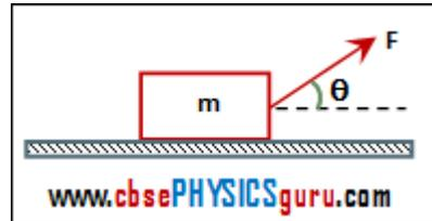
15. A horizontal force, just sufficient to move a body of mass 2 kg lying on a rough horizontal surface, is applied on it. The coefficients of static and kinetic friction between the body and the surface are 0.6 and 0.4 respectively. If the force continues to act even after the block has started moving, the acceleration of the block in  $\text{m/s}^2$  is (Take  $g = 10 \text{ m/s}^2$ ):
